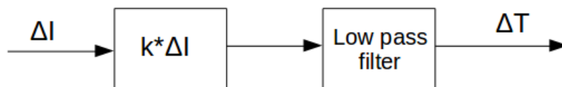
Figure 5: Flowchart for simple climate model. \Delta I is change in solar irradiance, and \Delta T is change in temperature.
